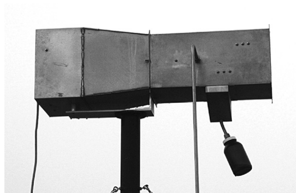
Fig. 1. The stainless steel Caltech Active Strand Cloud Collector (ss-CASCC).
