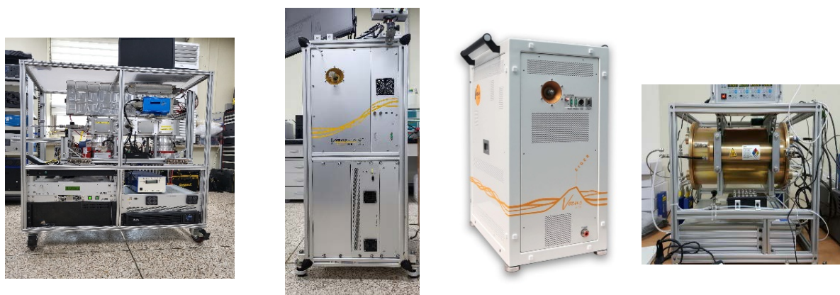
Figure 1. The AQL has real-time advanced measurement instruments for various research (HR-ToF-AMS, VOCUS PTR-ToF-MS, VOCUS-AIM (CIMS), OFR)
