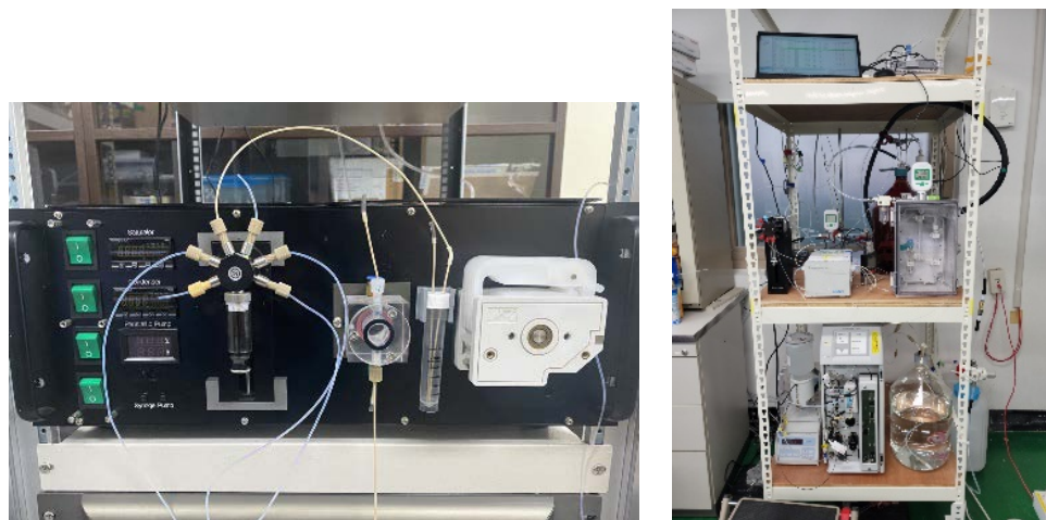
Figure 4. The AQL develops instruments (Particle Condensation System (PCS) for Aerosol and semi-continuous HNO 3 measurement system for atmospheric HNO 3 ).
